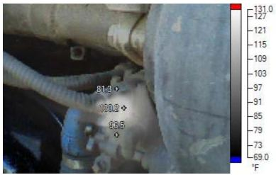
You can very quickly see proper heater operation and note that heat is properly being conducted into the blow down valve itself.
