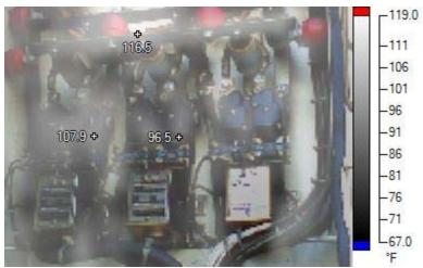
In this image you can see the general heat increase when the cooling fan test is in progress. This again gives a very quick indication of the relative state of the wiring and contacts, which in this case shows no major problems.
