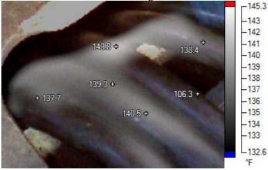
3. Contactors and relays high resistance contacts and/or connections. A general look with a thermal imager in any electrical cabinet under loaded conditions on the contactors or relays. To demonstrate this attached is a thermograph of cooling fan contactors on an SD60 unit with fan test engaged.
