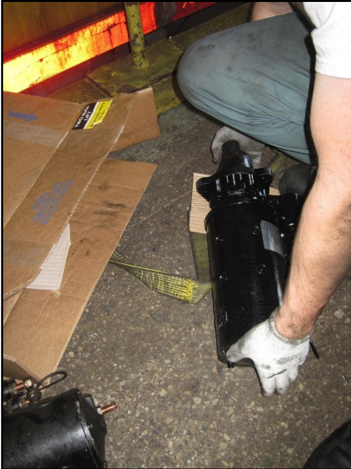
Starters Often Rolled From Box Onto Floor To Facilitate Strapping
