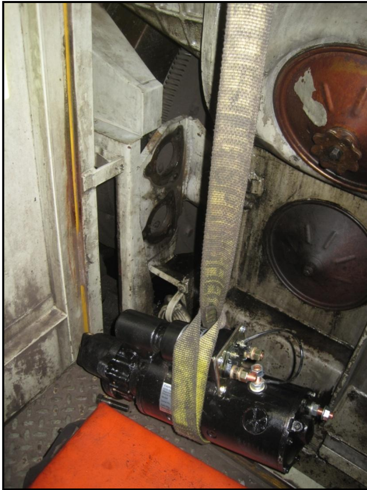
Starter Pushed Into Car Body And Aligned In Starter Bracket
