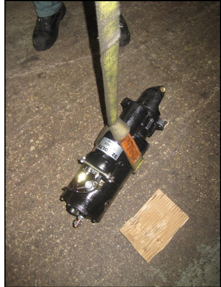
One End Picked Up Off Floor To Get Lifting Strap Around Starter and Solenoid
