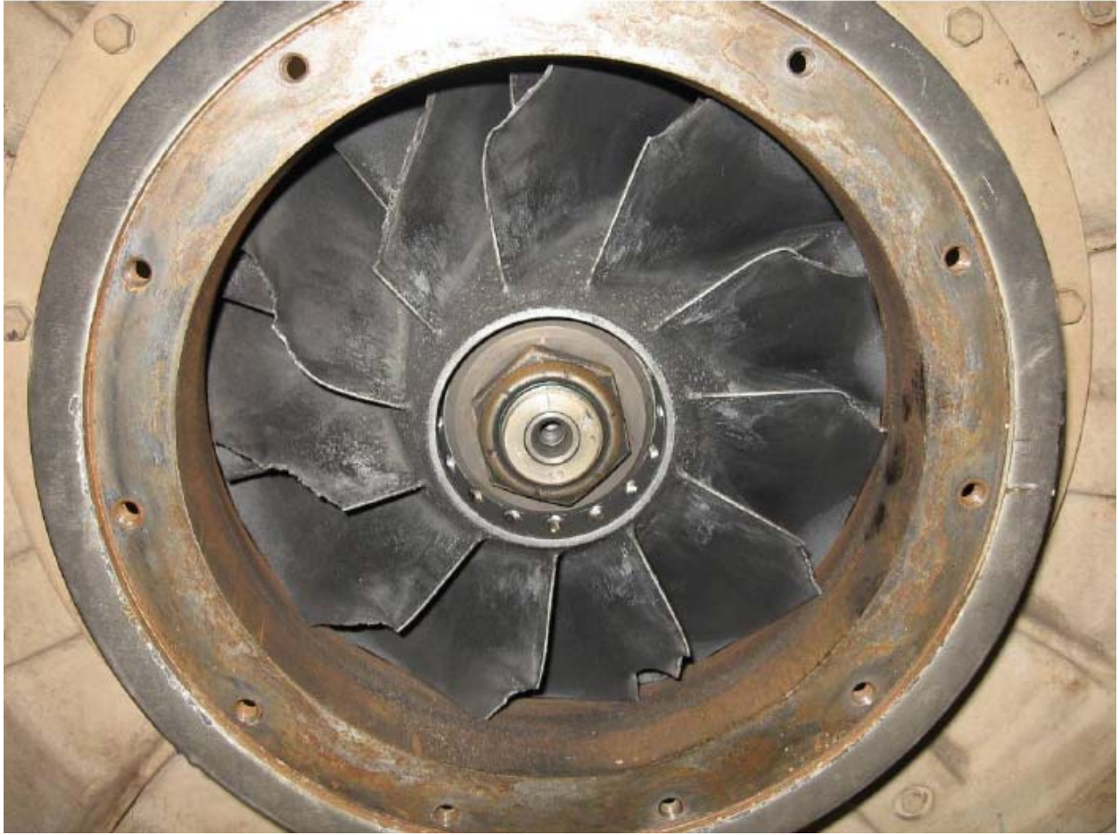
Figure 2 Impeller damaged due to foreign material ingestion
