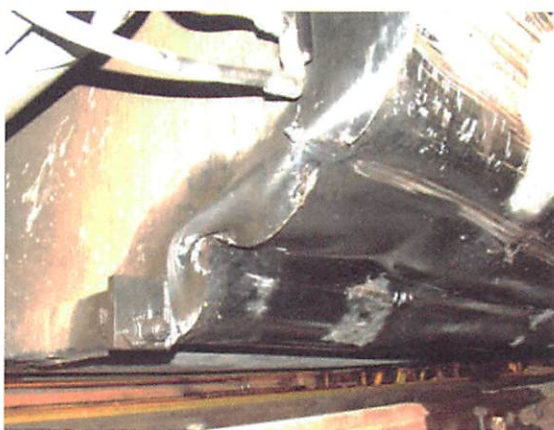
Fuel tank damage
