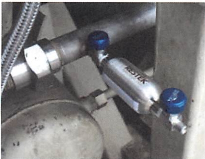
Figure 5 - Gas Sample Bottle Collection on Locomotive
