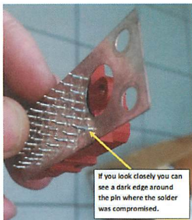
Figure 8. CMU Base with a Compromised Solder Joint
