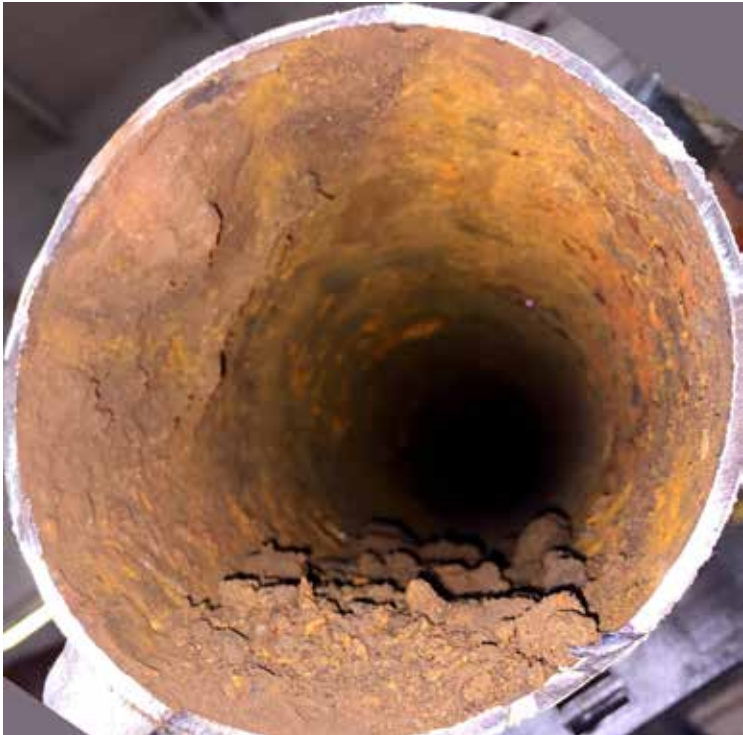
Figure 6. Corrosion Inside GE FDL Water Header Shown in Figure 5
