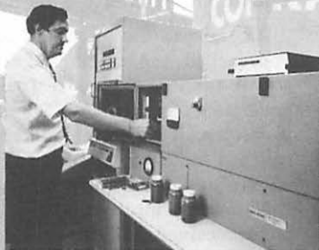
Conrail's Dan Reh runs Baird Spectrometer engine wear tests in the Selkirk, N.Y., facility, one of the system's five in-yard laboratories.
