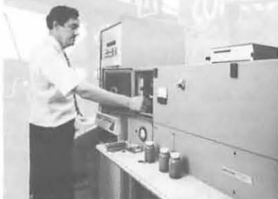
Conrail's Dan Reh runs Baird Spectrometer engine wear tests in the Selkirk, N.Y., facility, one of the system's five in-yard laboratories.
