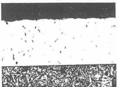
Metallographic Section of #2 Chromium Plate on Cast Iron Fig. 17
