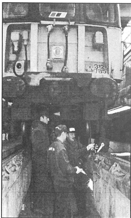
Figure 12: In-situ EMA inspection
