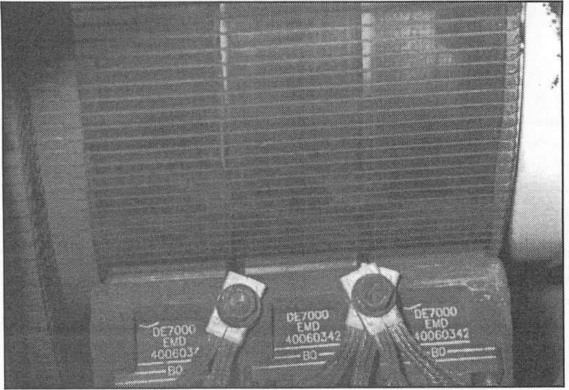
Figure 1: Commutator with high wear and TIR
