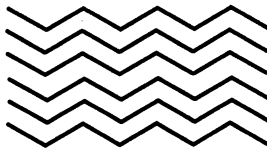
Without PPD Regular-shaped wax molecules form large crystals
