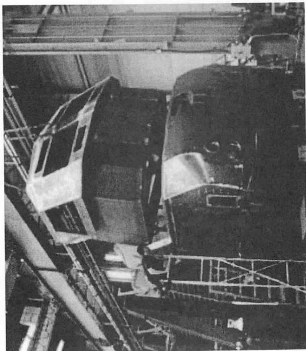
Cab structure and structural testing Figure 2
