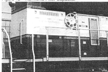
Engineer's Side view of Battery Box/Handbrake Area
