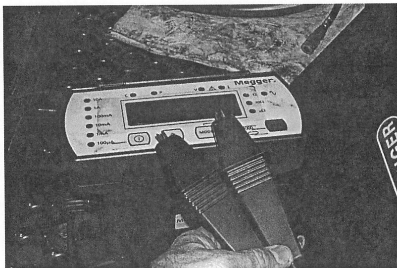
Figure 15 - Megger DLRO Low Resistance Ohmmeter
