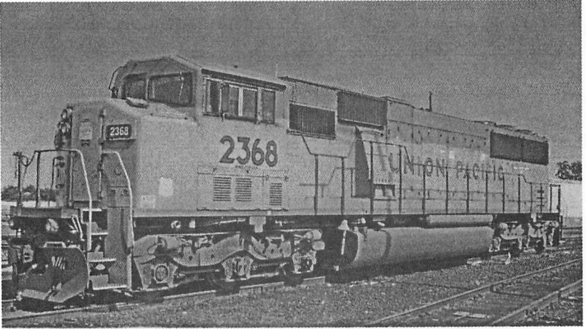
Figure #17 SD60 Line Haul Locomotive Fitted With Experimental DOC System
