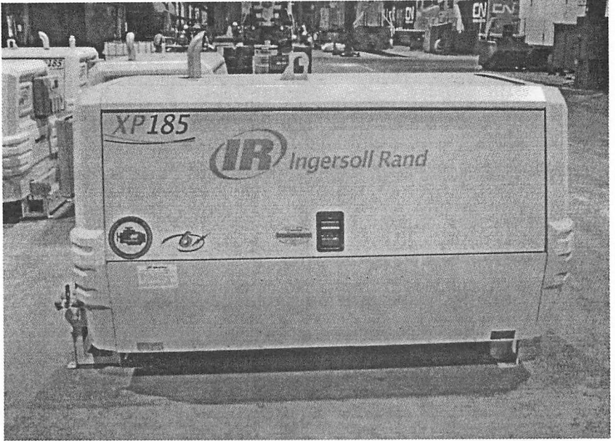
Ingersoll Rand air compressor w/6kW generator
