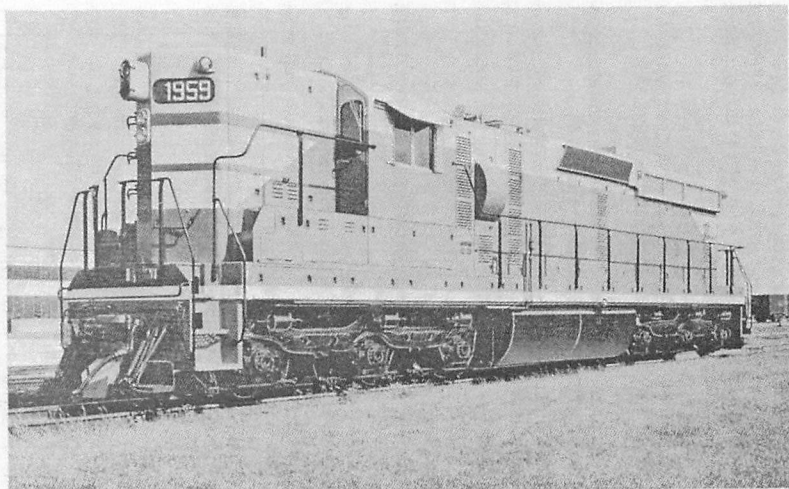
Figure 1 - EMD SD24 Locomotive of 1959 (from EMD Service Manual)
