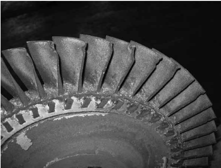
Figure 4: Foreign material damage to turbine wheel
