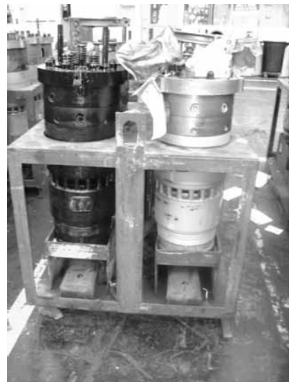
Power Assembly Rack
