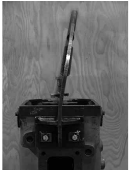
Power assembly lifter Rated Load of 1050 lbs Proof Tested at 2100 lbs Load Applied - Unknown
