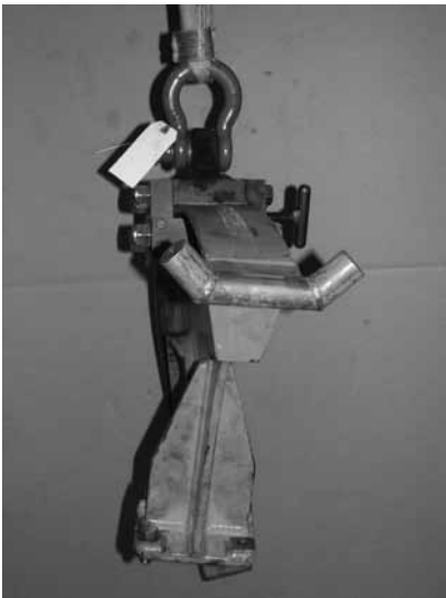
Power assembly lifter Rated Load of 1250 lbs Proof Tested at 2500 lbs Load Applied - Unknown
