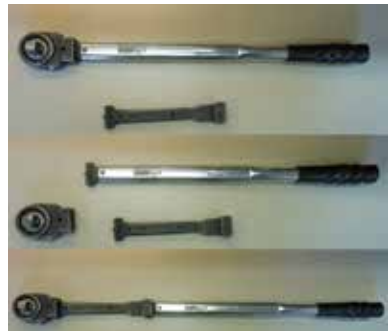
Figure 10 : Adding an Extension
