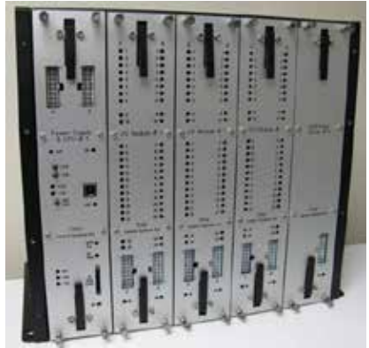
Figure 6 – TMV TECU locomotive control system
