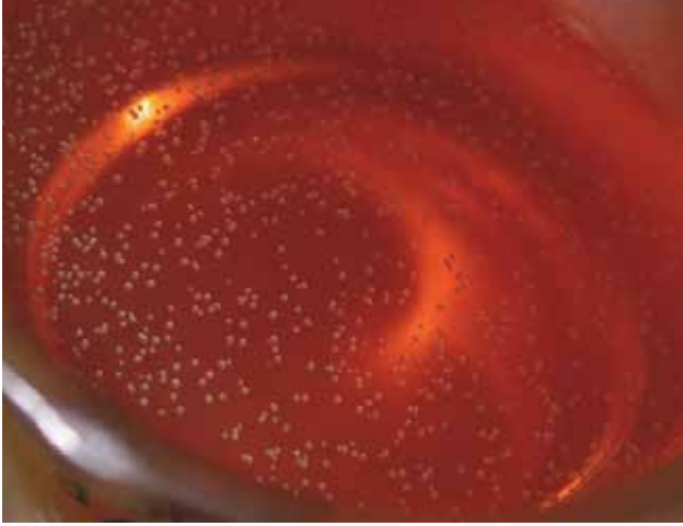
Figure 4: Additional images – Filter Plugging 2011-2012: Monoglyceride crystals beginning to form in B100 biodiesel after being held at 40F for 3 days
