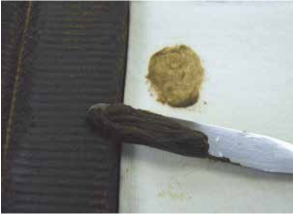
Figure 6: Pasty residue recovered from plugged filters. Analysis revealed mainly palmitate (C16:0) and stearate (C18:0) monoglycerides.
