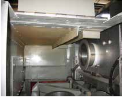
Figure 6: DPF Clean-out Access – Exhaust Connection to DPF Not Installed
