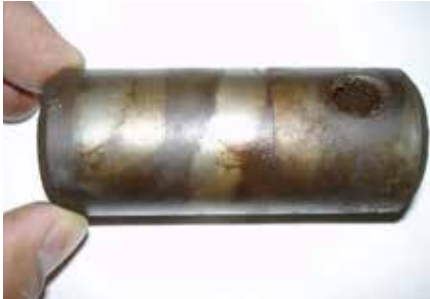
Brake Head Assembly Pin with 1,000,000 miles of service (SD70)MAC
