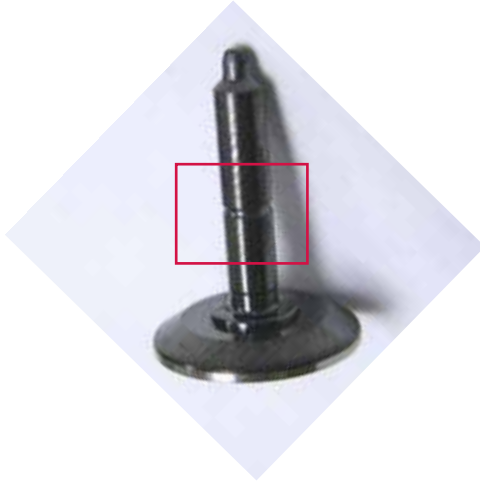
Figure 8: HPCR Injector with sticking pilot valve
