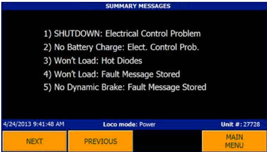
Figure 5. Modernized replacement for DID panel
