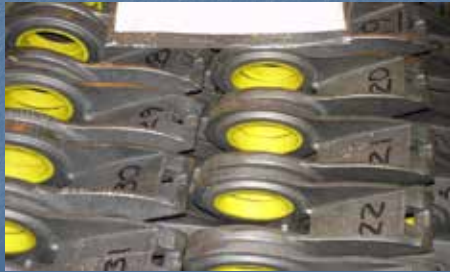
Complete Brake Head Assembly (GP38-2)
