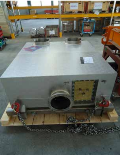
Figure 3: Front of DPF – Note Exhaust intake in Middle, Clean Out on Right Side and Exhaust Out at the Rear
