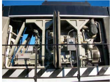
Figure 4: Engine and DPF Support in Car Body
