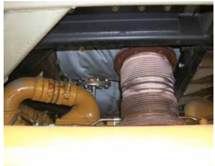
Figure 19: Exhaust Connection to DOC/SCR
