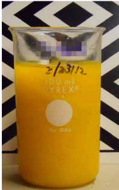
Figure 5: – end result, B100 held at 40F for 3 weeks. 40F was far above the classic 'cloud point' of the fuel
