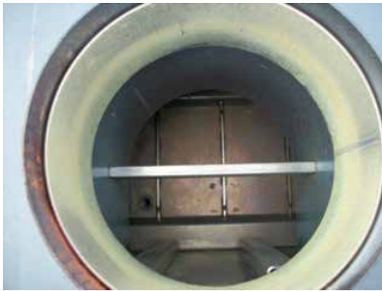
Figure 15: Exhaust Stack after 5,083 Hours
