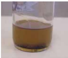
Figure 11. Wet, Dirty (Particulate) Diesel Fuel
