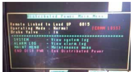
Figure 5: Remote DP screen showing Comm Loss
