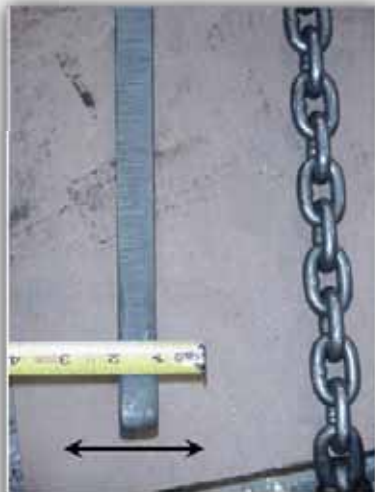
EXAMPLE OF HOW TO MEASURE LATERAL MOTION
