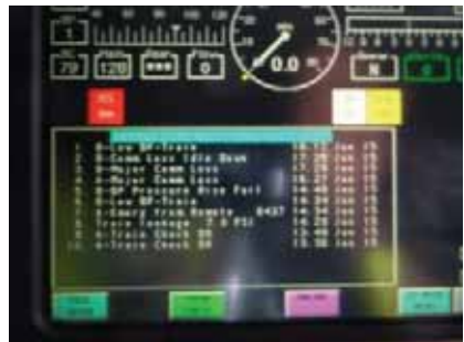
Figure 9: Low Brake Pipe Message
