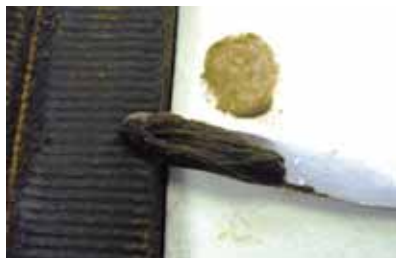
Figure 15. Metal Carboxylate Soap Plugged Filter
