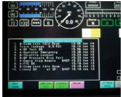
Figure 4: System Log showing "B-Comm Loss Idle Down"
