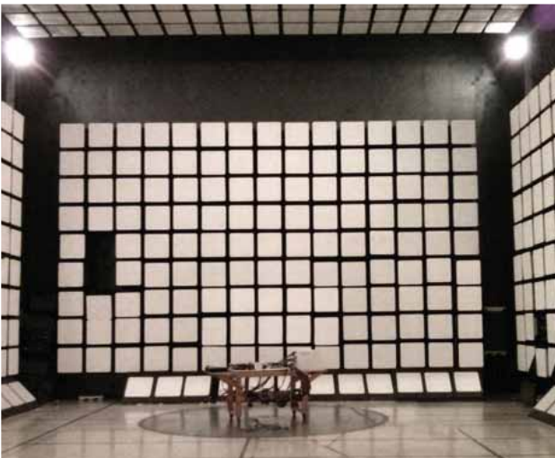
Figure 7: EE during Conducted Emissions Test
