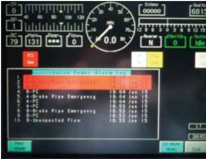
Figure 10: Active and Inactive Brake Pipe Emergency messages
