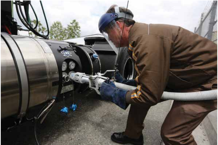
Figure 8 – LNG Refueling Hose and Protective Equipment
