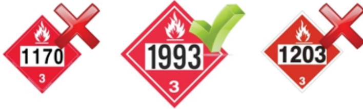
Figure 1. Proper Diesel Fuel Placard
