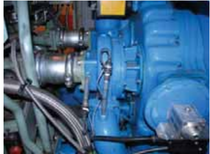
Figure 10 – Cable strain relief improvement
