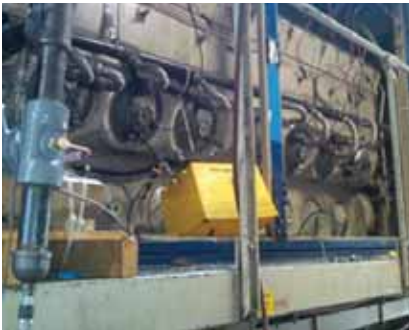
Natural gas port injection on an EMD engine (test unit)
