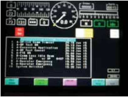
Figure 13: Loss of serial communication on lead
