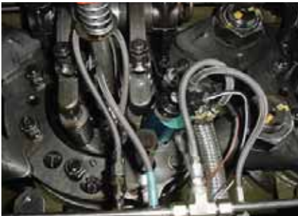
Dual Injector Installation
