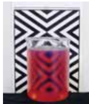
Figure 7. Wet, Hazy Diesel Fuel
