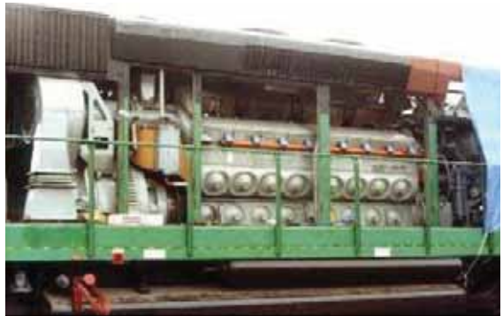
Dual fuel installation in an EMD locomotive
