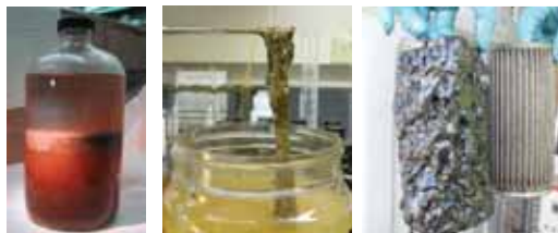
Figures 8-10. Diesel Fuel and Filter with Microbial Contamination
