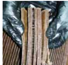
Figure 14. DRA Plugged Filter
