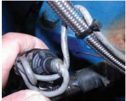
Figure 8 – Water pressure transducers, cable twisted
