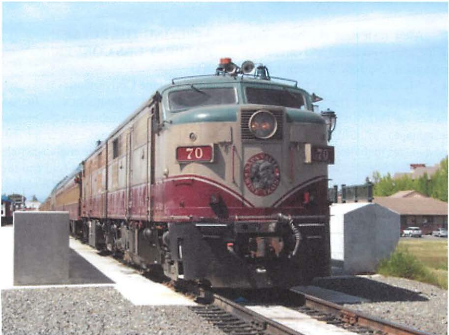
Figure 2. Napa Valley Wine Train FP4 Locomotive with natural gas 645E engine.
