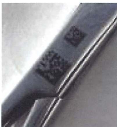
Figure 5: Example of Laser Bar Code on tool
