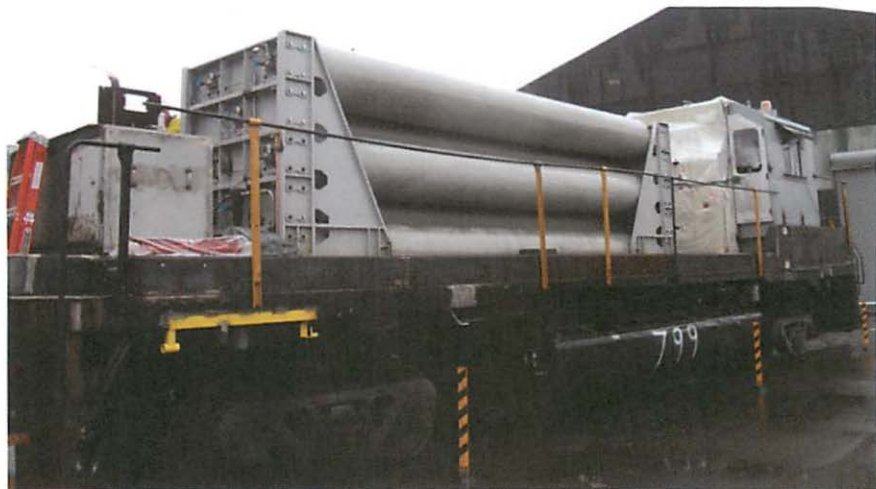
Figure 1. NS 799 RP-E4C slug under construction showing the natural gas cylinders.
