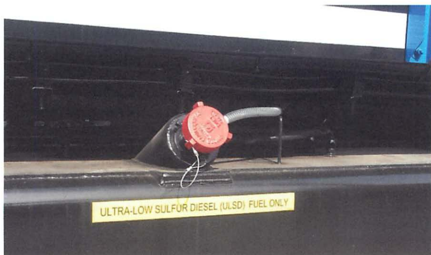
Figure 3. Example of Tier 4 Locomotive Fuel Labeling
