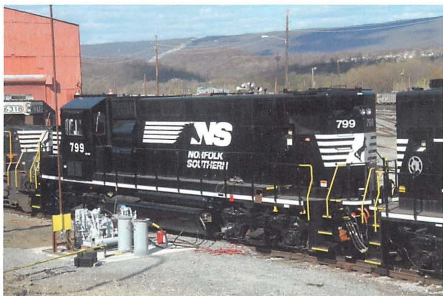
Figure 9. NS RP-E4C Natural Gas Slug
