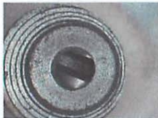
Bore Hole Access port for 4mm borescope
