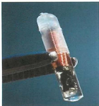
Figure 7: RFID device for implanting into animals
