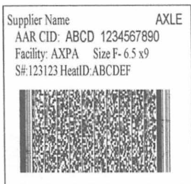
Figure 2: AAR S-290 Sample Axle (with CID) Bar Code
