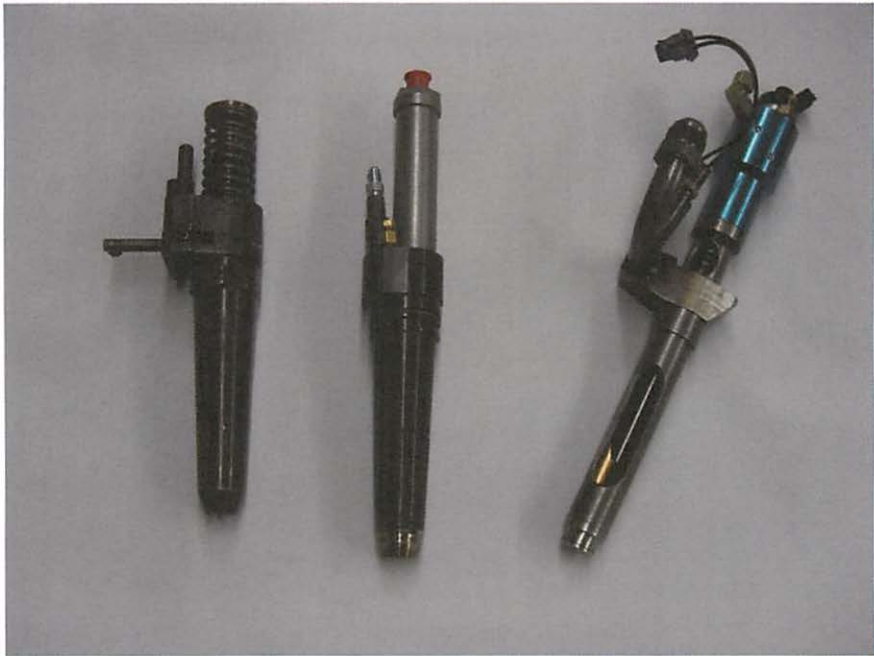
Figure 7. Diesel Injector (left), Pre-Ignition Chamber (middle), Gas Injector (right).
