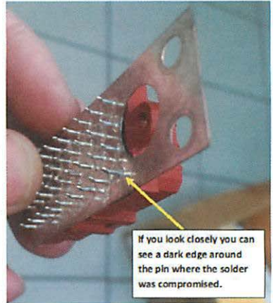
Figure 8. CMU Base with a Compromised Solder Joint
