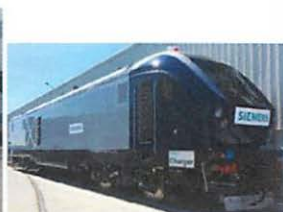
Siemens SC-44 Charger 2016 Cummins QSK95 Siemens IGBT AC Traction & HEP Customer: IDOT/Multi-State
