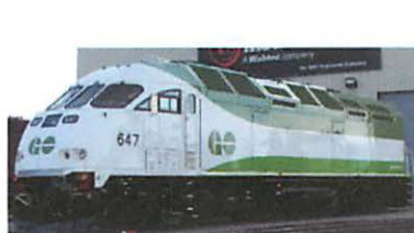
MPI MP54AC 2016 Twin Cummins QSK60 ABB IGBT AC Traction & HEP Customer: GO Transit
