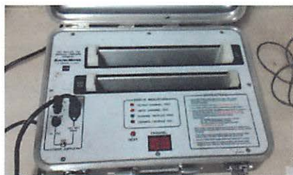
Figure 7. EMD DIO Bench Tester
