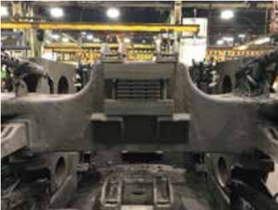
Nose Pack on Dash 9 DC Truck Frame
