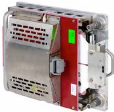
Figure 13: Water cooled power core from CAF Power&Automation. (Used with permission.)
