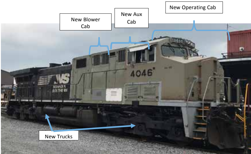
Converted Locomotive prior to Paint
