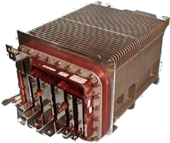
Figure 7: Siemens GTO inverter, used in the original EMD AC traction locomotives. (Used with permission)
