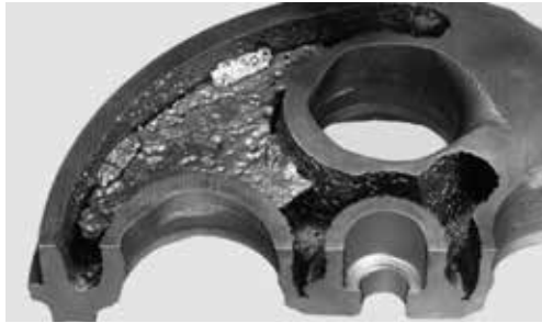
Buildup of scale on a cylinder head fireface.
