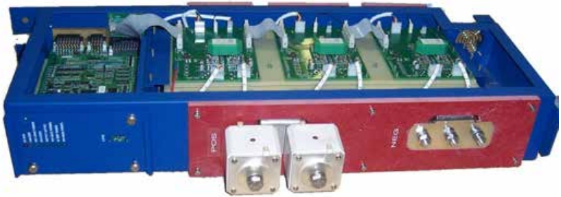
Figure 14: Liquid cooled inverter from American Traction Systems. (Used with permission)
