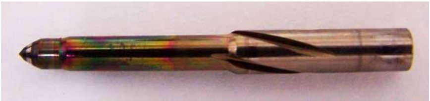
Figure 6—Lacquer Type Injector Deposit (Innospec Fuel Specialties)
