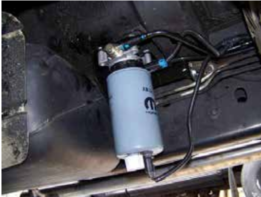
Figure 9—Mopar Severe Fuel Filter System Mounted on Fuel Tank Bottom
