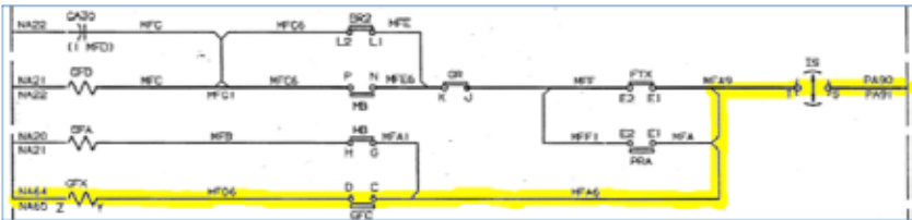
Figure 1. Example GFX circuit on a SD40-2 locomotive
