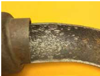
Erosion/corrosion of a water jumper
