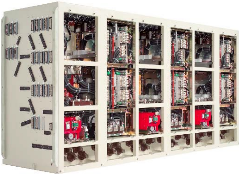
Figure 2: Traction inverter cubicle from Siemens' DC to AC conversion on electric locomotives in Australia. (Used with permission.)
