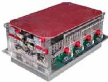
Figure 10: An example of an air-cooled power core from CAF Power&Automation, based in San Sebastian, Spain. (Shared by permission of CAF Power&Automation.)
