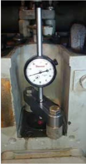
Figure #10 Measurement System Installed in Place of High Pressure Fuel Pump
