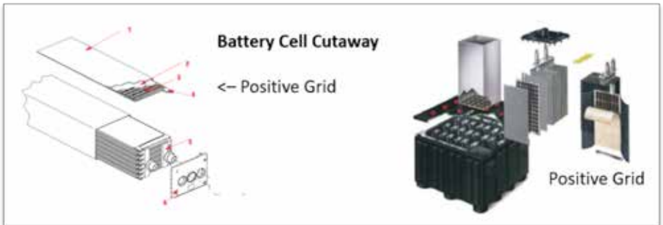
Figure 8 - VRLA and Flooded Lead Acid Cell Cutaways
