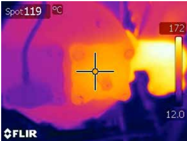
Figure 4 – F40, engine injection system thermal analysis
