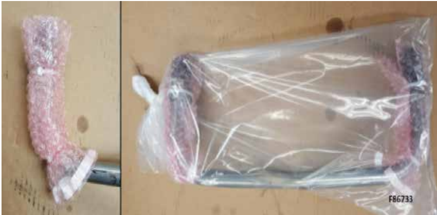
Example of clean packaging and bubble wrap application.
