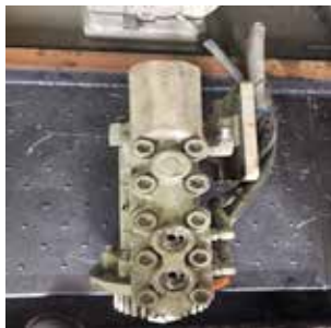
This High-Pressure pump was left open the shop atmosphere; no plugs.
