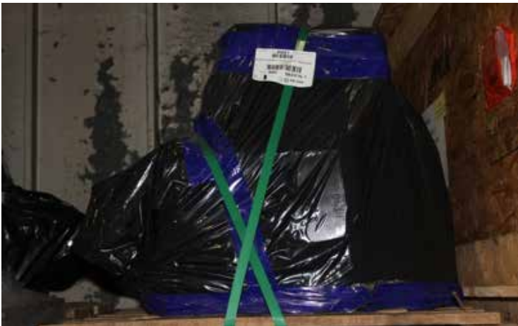
An OEM head wrapped from the factory. It is wrapped, taped and bound to the pallet to eliminate the chance of contamination.
