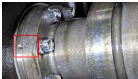
Figure #6 Cam Timing – Aligning the Cylinder Marker and the Notch in Cam Journal
