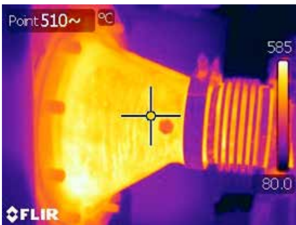
Figure 3 – EPA-42, engine injection system thermal analysis
