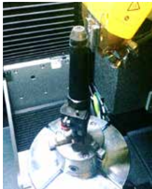
Figure 9. EMD 645 Fuel Injector mounted in the CT scanner for high-resolution scanning of the tip.
