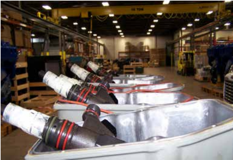
Fuel injectors open to shop air contamination. Note that ports into the injector are not plugged.
