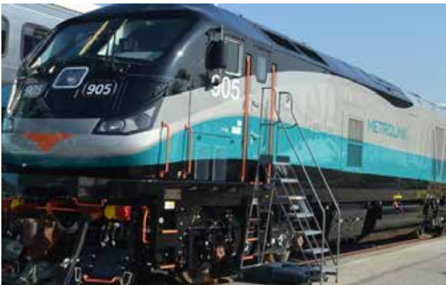
Figure 13 EMD F125 Passenger Locomotive
