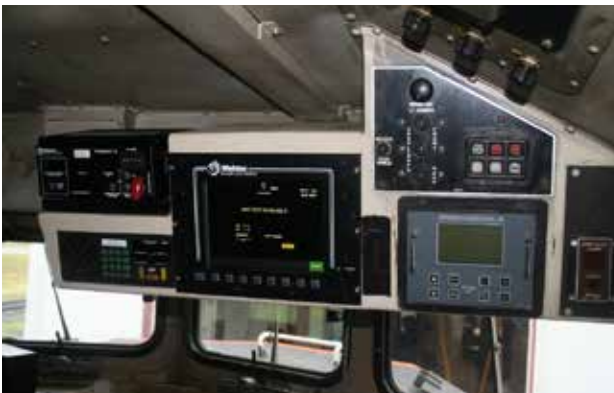
Figure 5: In cab PTC equipment that must typically be installed in each locomotive.
