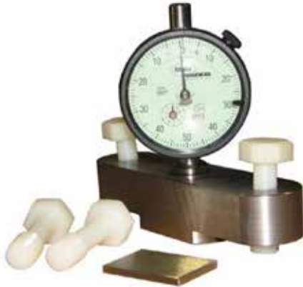
Figure #14 Standard TESCO Part Number T55971 Used to Set Fuel Pump Push Tube Height https://tescotools.com
