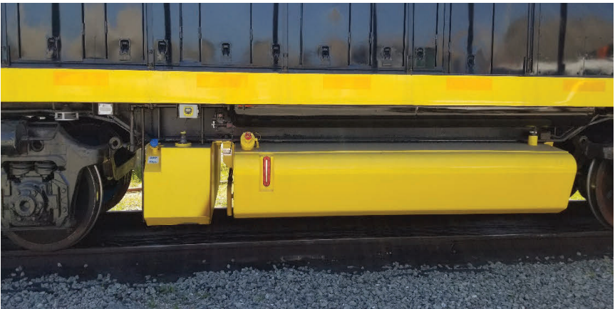
Figure 5: Locomotive DEF Tank
