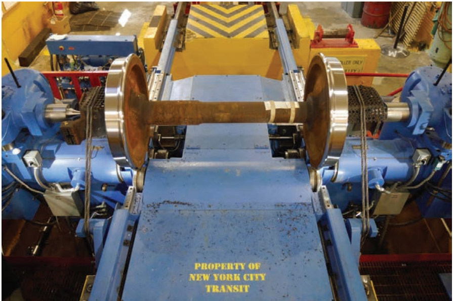
Wheel truing machine clamping process
