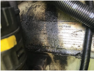
Oil Soaked 7FDL Engine Plate
