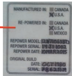
Filling in the Information on the EMD Repower Label with marker
