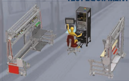
DOOR SYSTEM BENCH TEST EQUIPMENT
