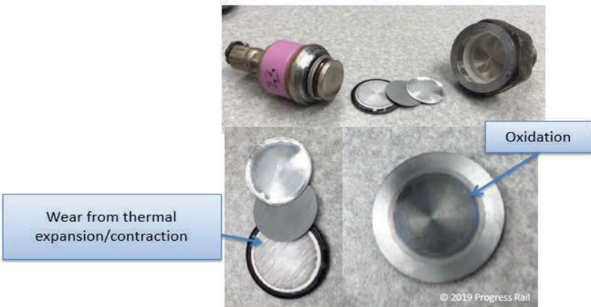
Figure 9. Disassembled aged diode showing wear.
