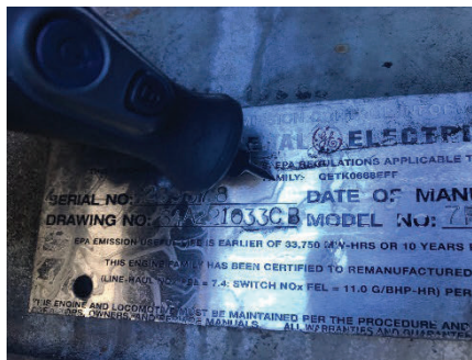
Scribing the Date Character on the GE Engine Label
