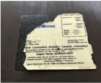
Deteriorated and Damaged EMD Label
