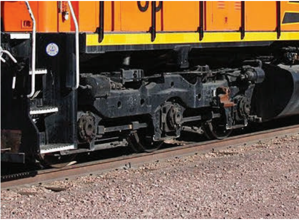
Friction Bearing Journal Box - This bearing typically consists of lead babbitt over a brass bearing shell.
