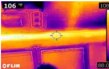
Figure #16 Temperature delta between insulated and non-insulated area = 20°F (88°F to 108°F)
