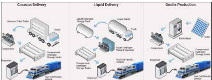
Figure 8: Hydrogen Fueling Station Examples
