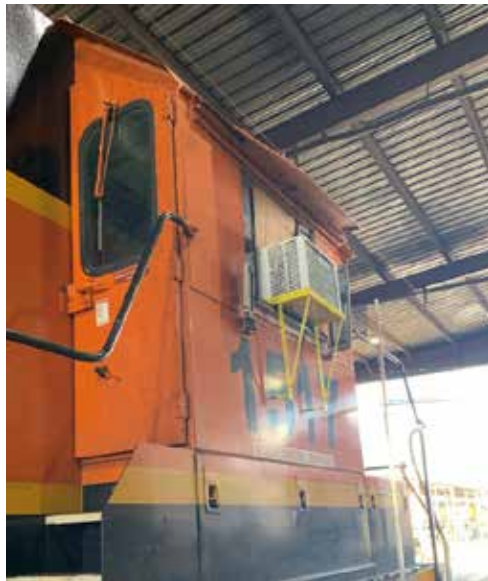
Picture 5: Artisan cab cooling system
