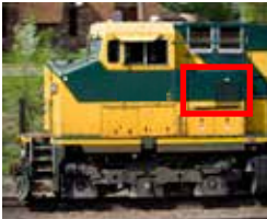
Figure #4 GE Dash 8, Dash 9 cab with Sidemount HVAC System
