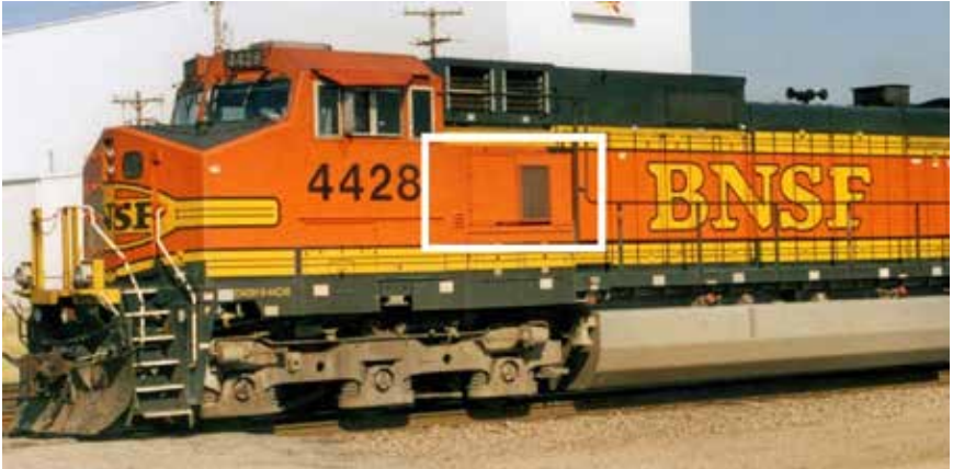
Picture 6: GE Side Mounted HVAC
