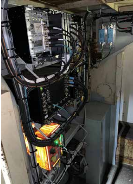
Picture 2: PTC and latest electronic hardware installed in a short nose
