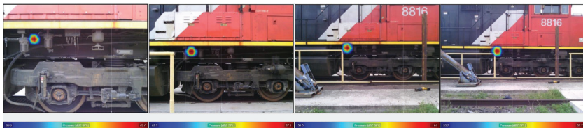
Figure 2. Air Leak at 3.0, 4.5, 6.0, and 7.5 Meter Distances
