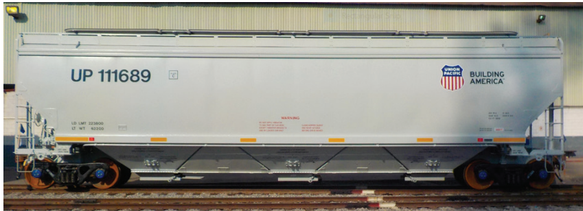
Figure 15 – Covered Hopper with Aerodynamic Modifications Installed
