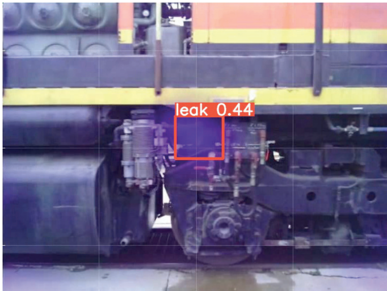
Figure 8. YOLOv5 Detection of an Air Leak
