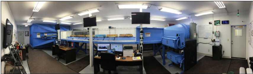
Figure 18 – Wind Tunnel configured for G scale (1/29th) model testing (now owned by MxV Rail in Pueblo CO)
