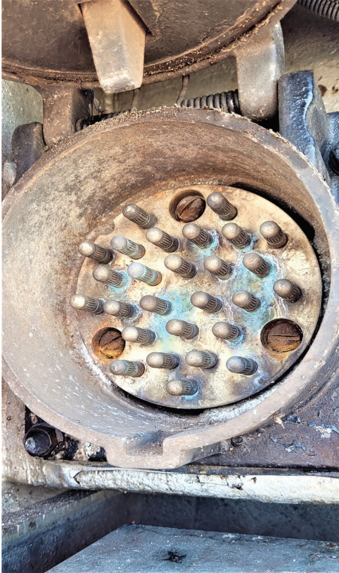
Figure 10: MU Receptacle Issue: Water Ingestion
