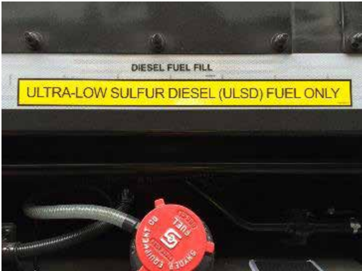
Ultra-Low Sulfur Diesel Fuel Label Required for Tier 4 Locomotives (including Tier 4 Credit Locomotives)
