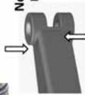
Non-alignment control lacks "wings" on shank at coupler pin
