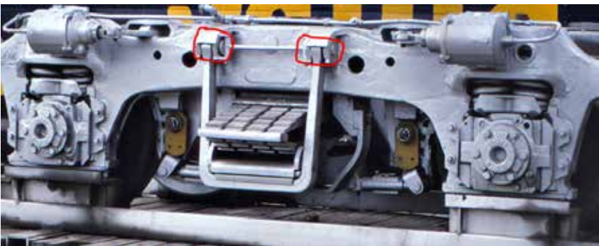
Figure 4 – Location of bushings on the swing hanger assembly on two-axle Blomberg trucks
