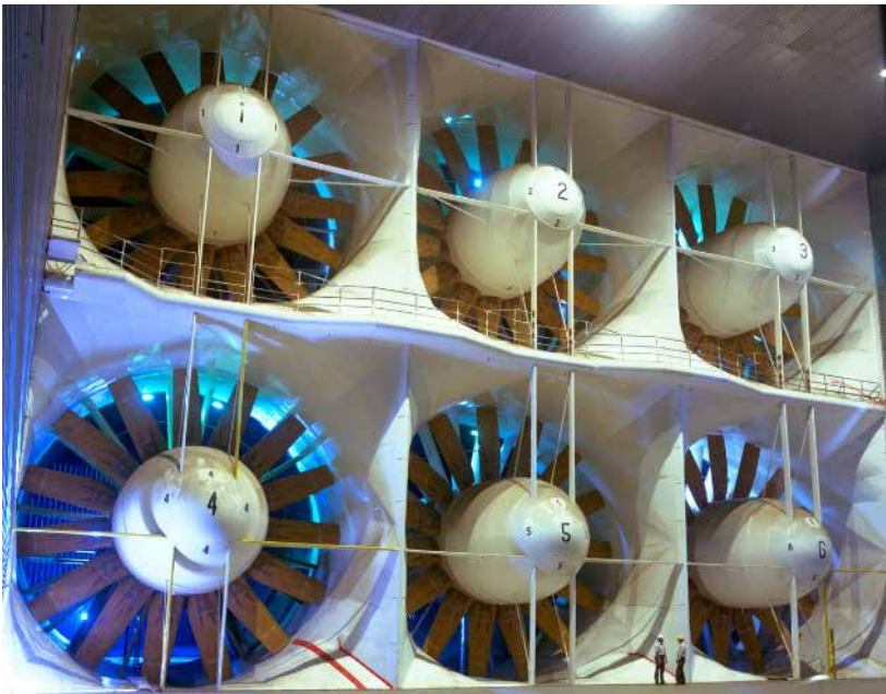
Figure 22 – Inlet Section of the Largest Wind Tunnel in the World at NASA Ames Research Center [27]
