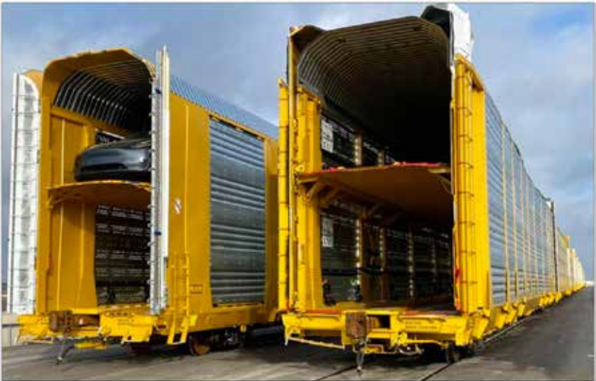
Figure 13 – Autorack Vehicles with Doors Open and Aeroscreens Installed on Sidewalls
