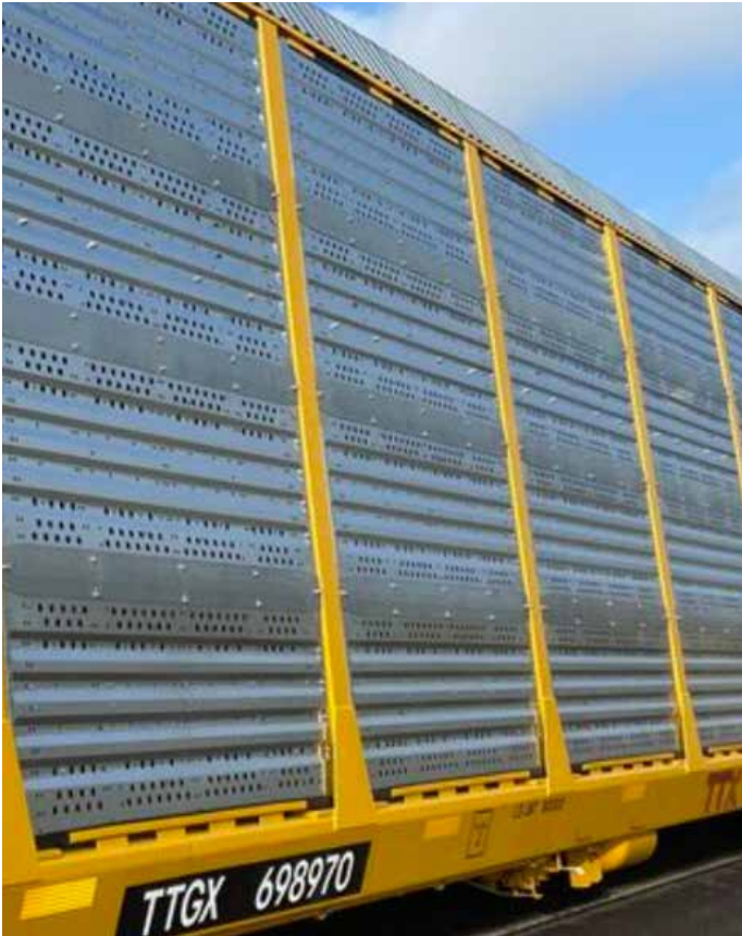
Figure 26 – Aeroscreens with a Modified Punch Hole Pattern [31]
