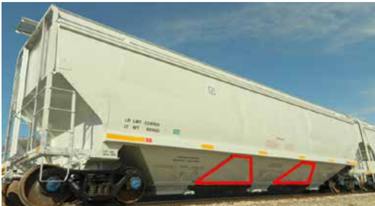
Figure 9 – Covered Hopper with Aerodynamic Modifications Installed (Red Outline Highlighted)
