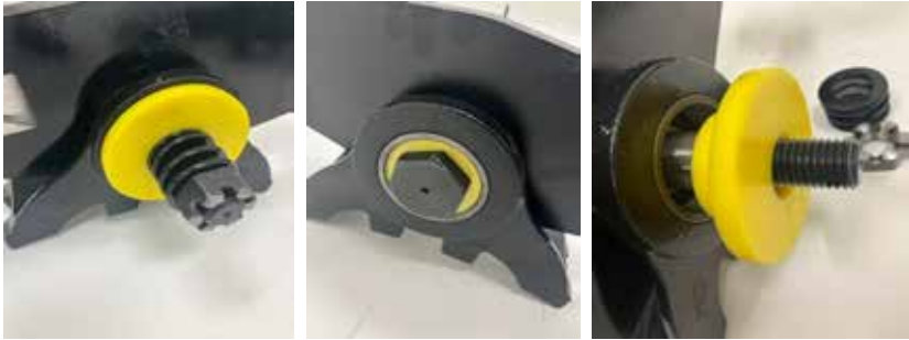
Figure 5 - GP Clasp; Outside Dead-Lever Brake Head Assembly Application
