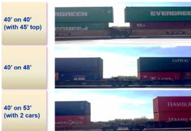
Figure 16 – Variance of Gap Size Between Top Container Wells
