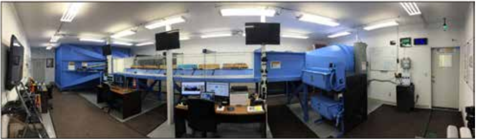
Figure 23 – Wind Tunnel Configured for G scale (1/29 th ) Model Testing
