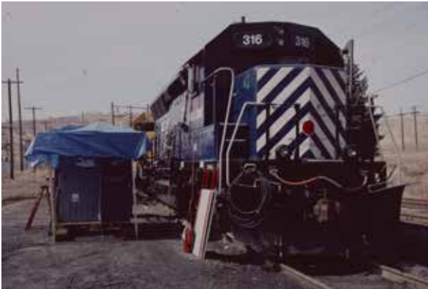
Figure 2. Connected SD45-2's Providing Synched Grid Power
