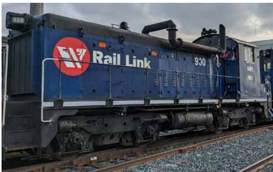
Figure 1: EMD SW900 switcher locomotive used in fuel-switching study. Custom exhaust system used for emissions sampling and exhaust flowrate measurement shown installed.
