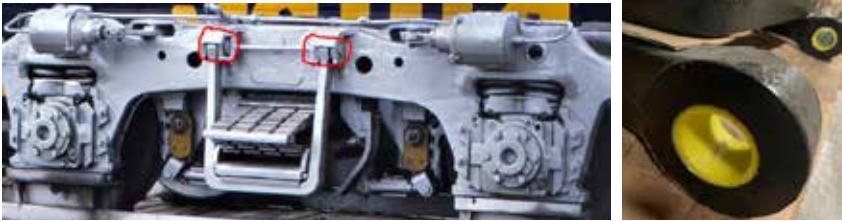
Figure 18 - Application of thermoplastic bushings in swing hanger
