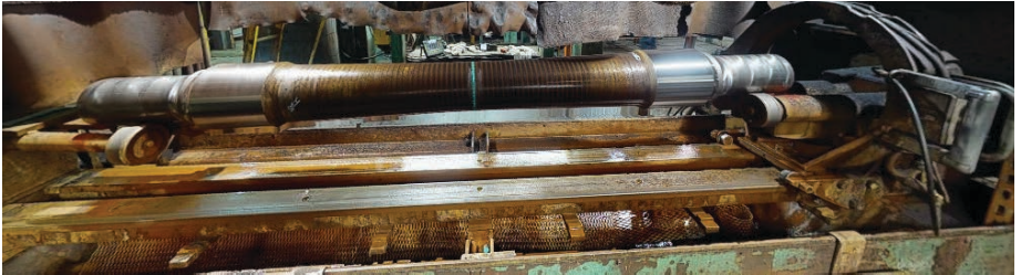
Figure 4 Axle Undergoing Magnetic Particle Station
