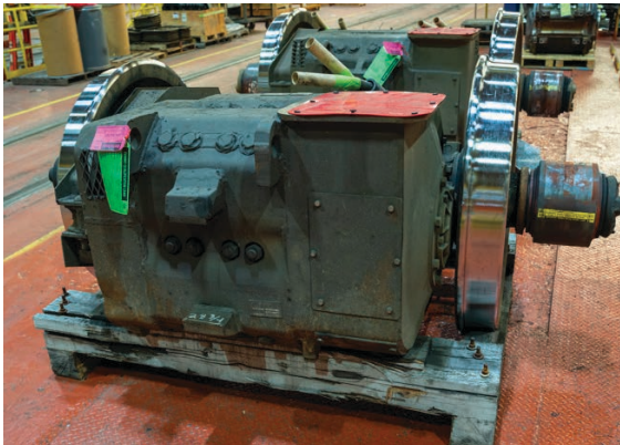
Figure 2 Locomotive Combo Units Post Inspection and Wheel Truing
