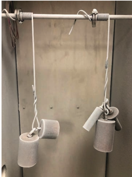
Figure 4. Cold Bend Mandrels and Cold Shock Test
