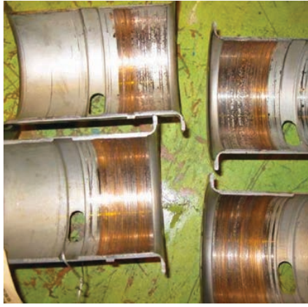
Figure 2: Damaged Cam Bearings
