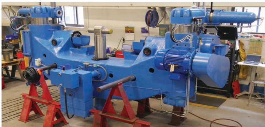
Figure 3 Remanufactured Stanray® Wheel Truing Machine
