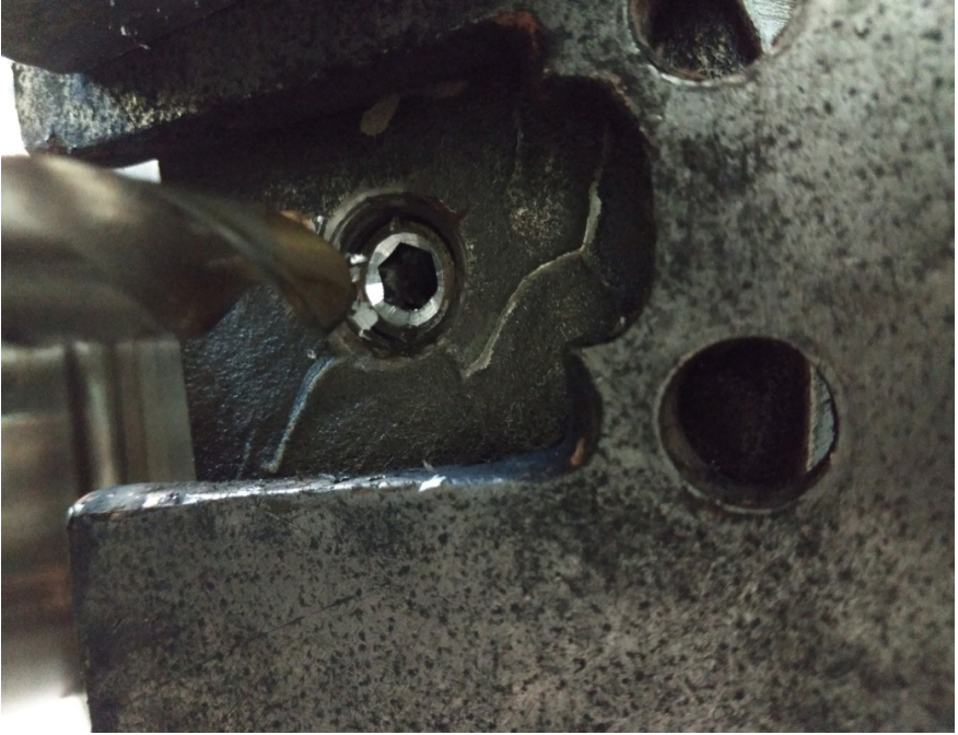
Figure 13 - Drilling the plug
