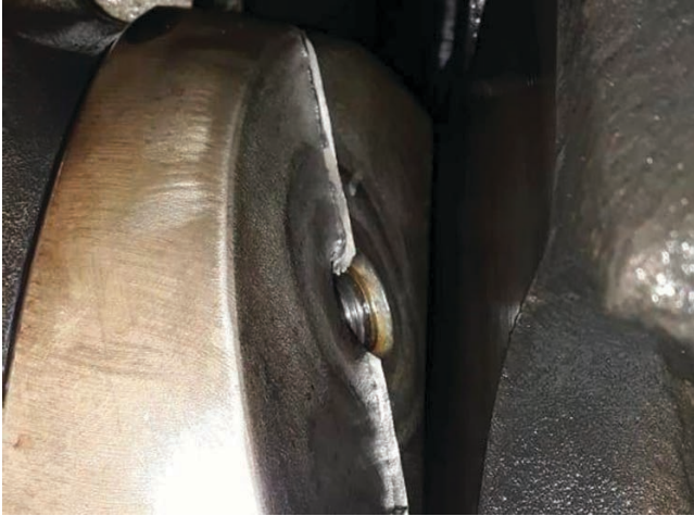
Figure 1 - Fractured crankshaft assembled
