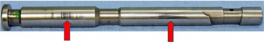
Figure 4: Scored plunger due to contamination
