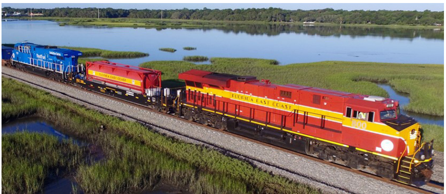
Wabtec (GE) Dual-Fuel Locomotives with LNG Tank Car Fuel Tender
