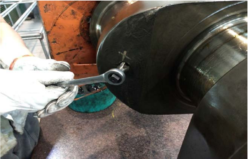
Figure 14 - Cleaning the thread with a threading bit
