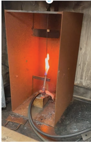
Figure 7. ICEA Vertical Wire Test
