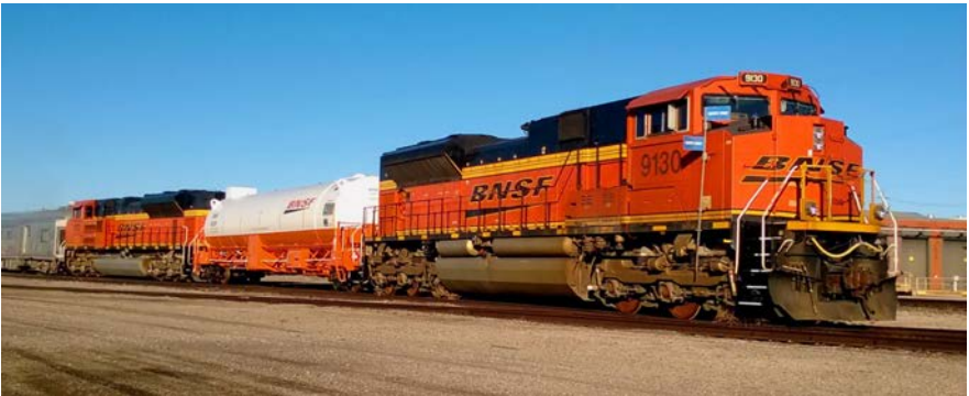
Progress Rail (EMD) Dual-Fuel Locomotives with LNG Tank Car Fuel Tender
