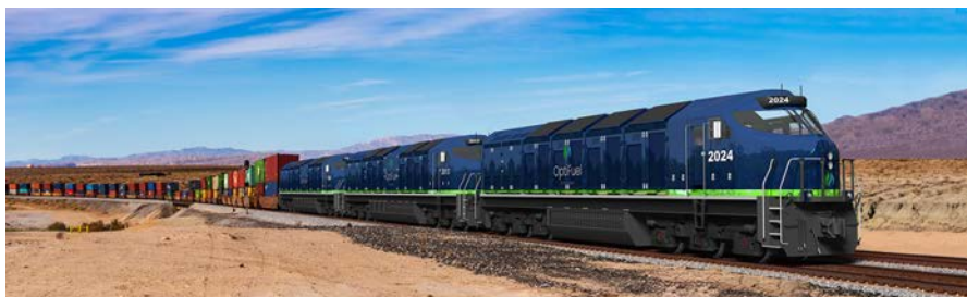
Artist Rendition of Proposed OptiFuel Dual Fuel Diesel/RNG Hybrid Line Haul Locomotive
