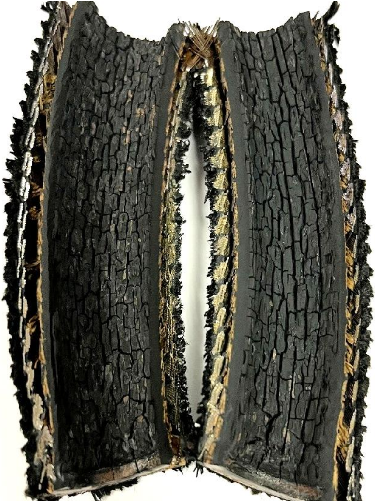
Interior of a rubber fuel hose is cracked and brittle after exposure to alternate diesel fuel blends.
