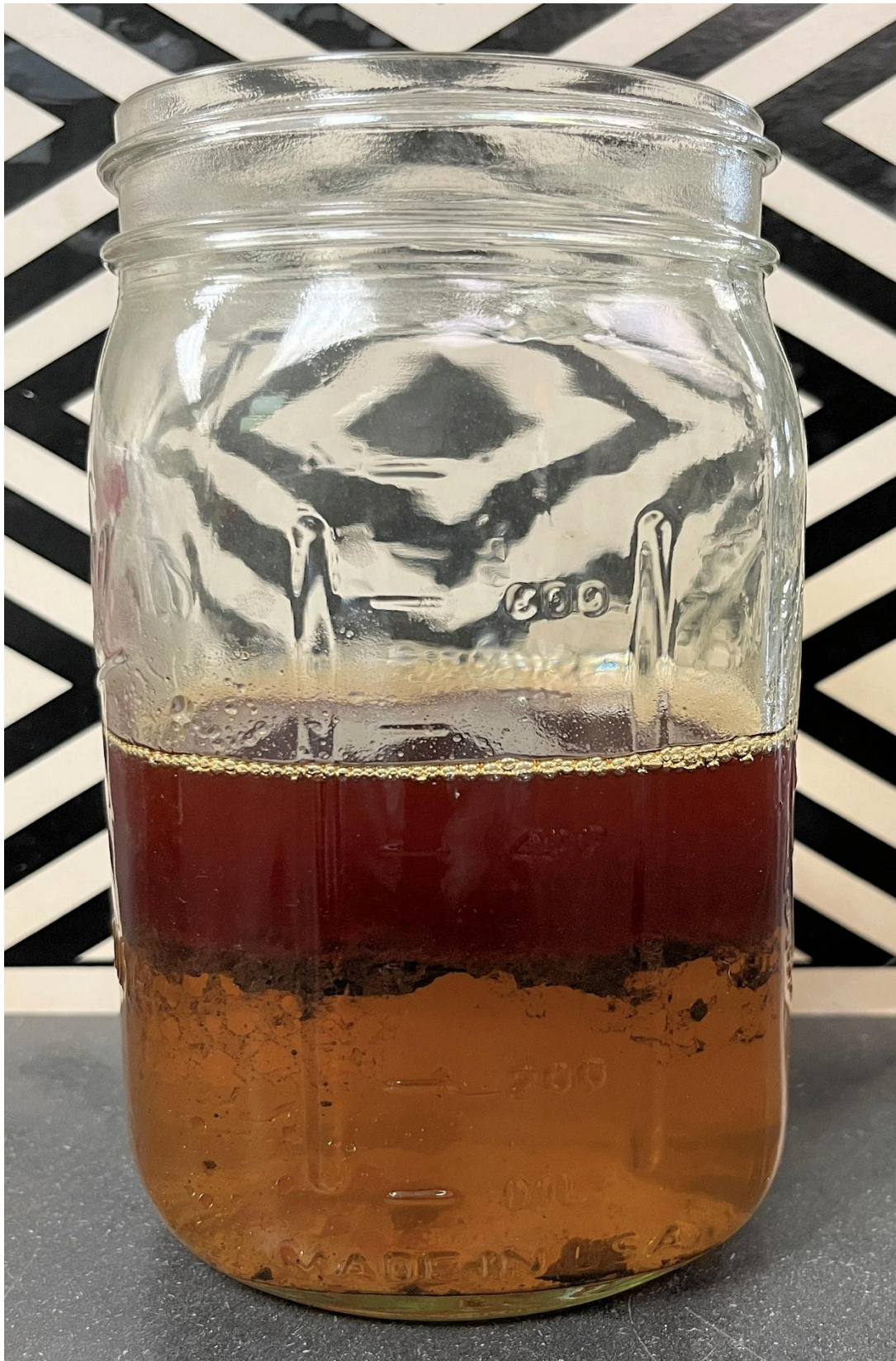
Fuel sample showing two distinct layers – rusty water (bottom), dull, red cloudy fuel (top). An intermediate brown/black 'rag layer' of biologic growth is also noted at the fuel/water interface.
