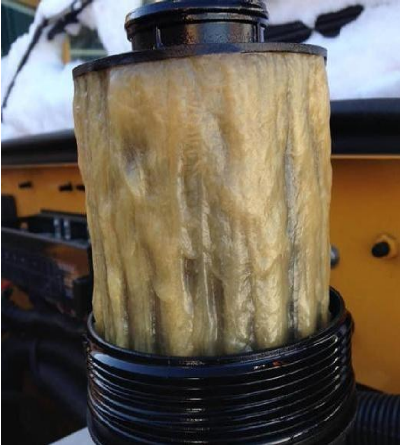
A fuel filter displaying a typical build-up of wax during a winter cold season.
