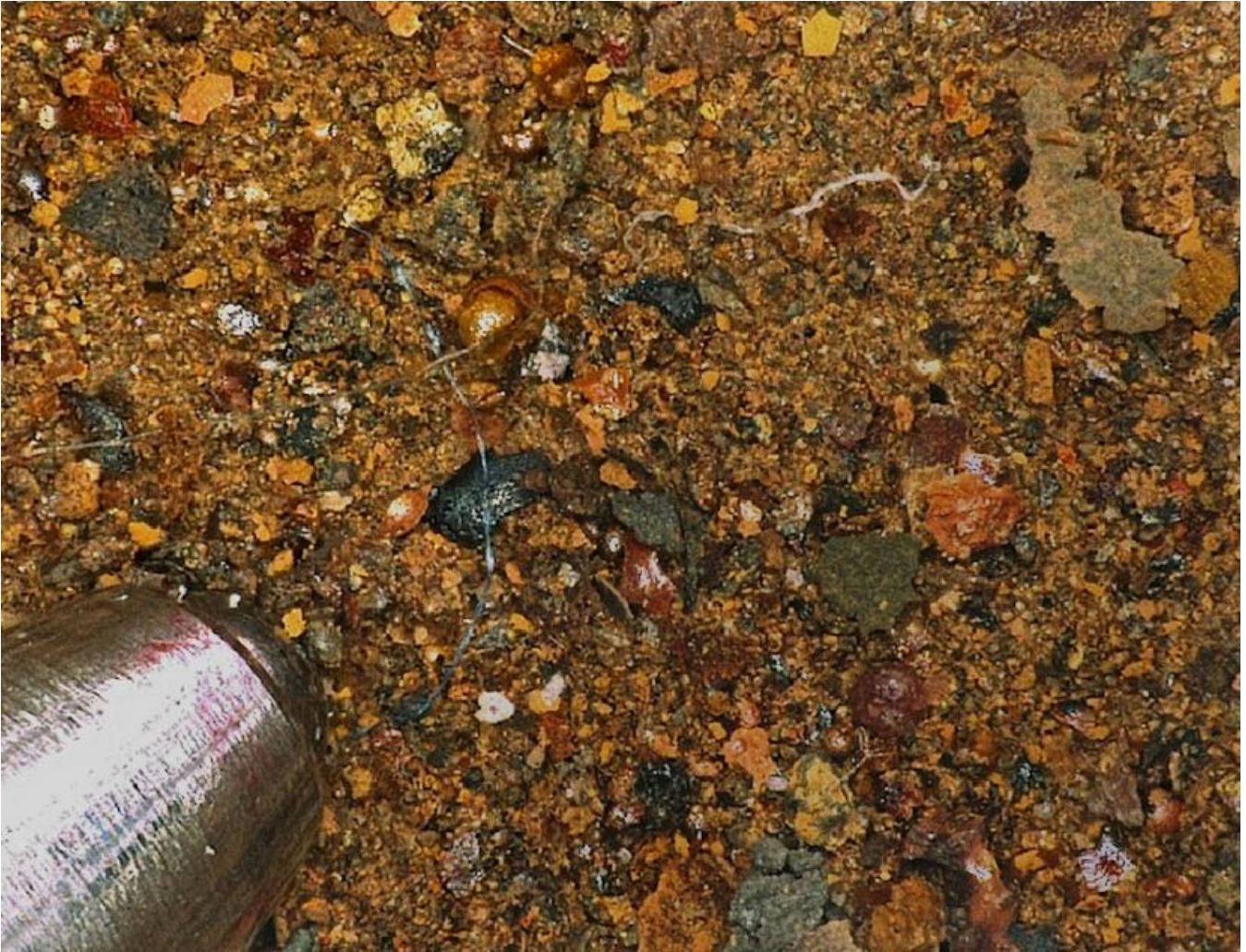
Rust flakes and other oxidation debris removed from a fuel filter. (Ball point pen, left, for scale)
