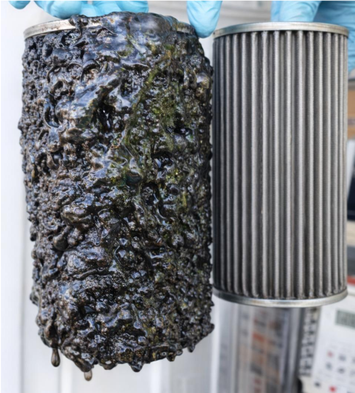
A fuel filter plugged with a bacterial colony (left). Typical new fuel filter (right).
