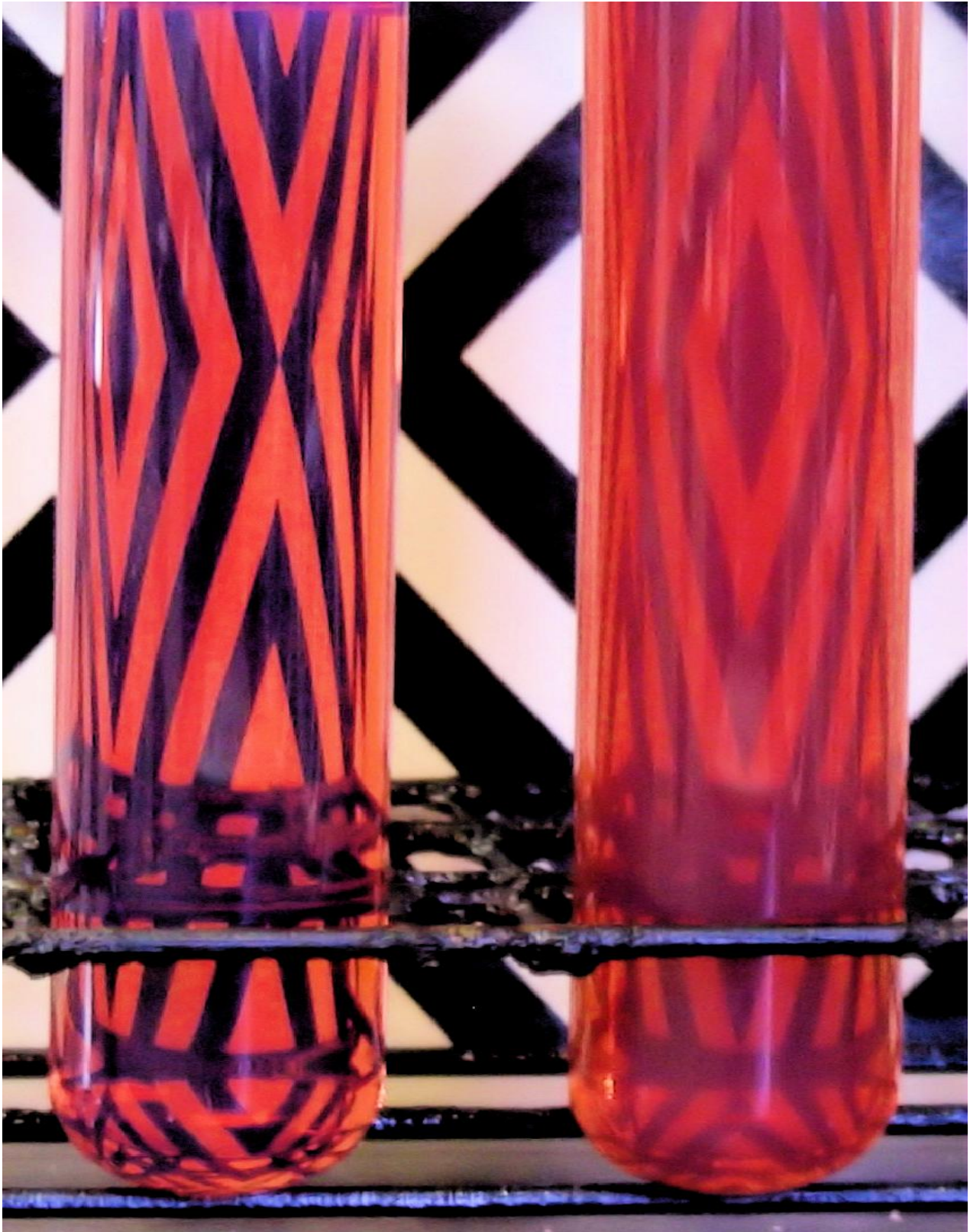
Typical “clear and bright” fuel sample (left). Cloudy sample with suspended water (right).
