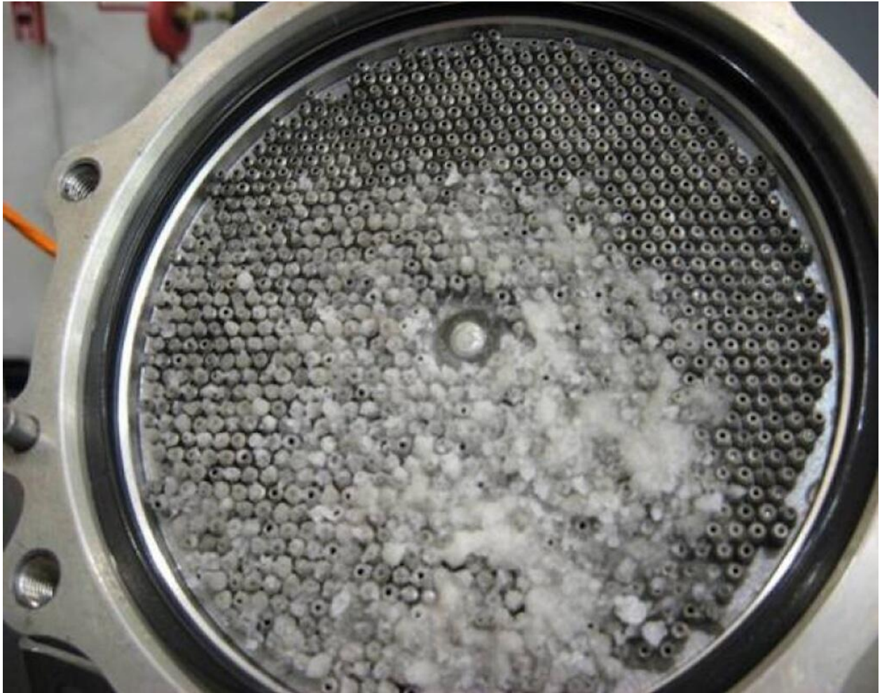
Image of ice accumulation on a fuel filter. Note the general lack of color and the ice appears mainly 'snow white'.
